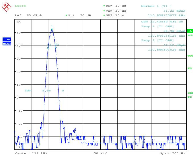
99% Bandwidth / 0.111MHz / WPT\_111kHz\_unmodulated
