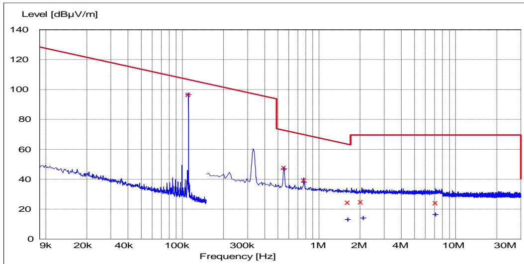
Quasi-Peak (< 150 kHz: RBW: 200 Hz, >150 kHz: RBW: 9 kHz)
