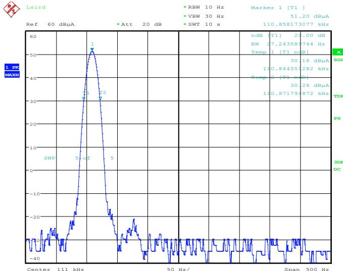
20dB Bandwidth / 0.111MHz / WPT\_111kHz\_unmodulated
