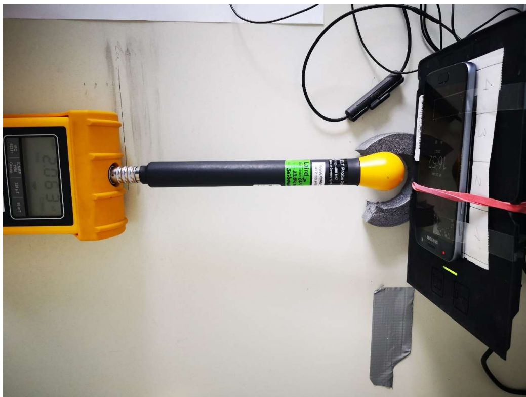
H-Field, worst case position, middle coil, 4cm
