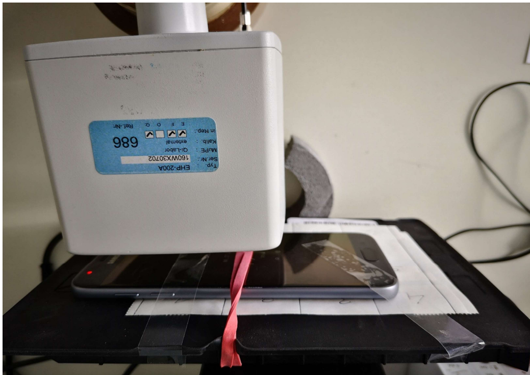
E-Field, worst case position, right coil, 4cm
