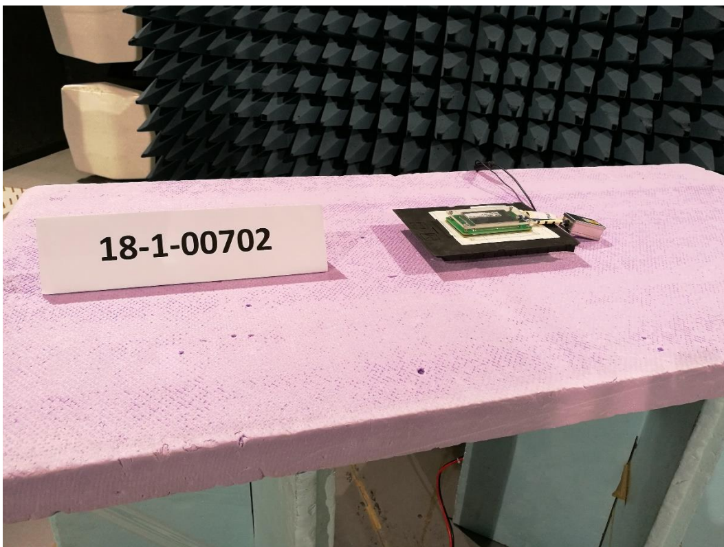
Photograph 4: close view of the setup in the semi-anechoic chamber
