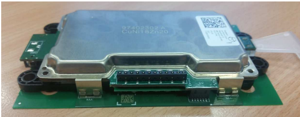
Main Board with shielding + Cap Sensor Board + Coil Module (mounted)
