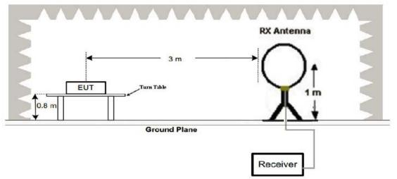
(2) Radiated Emission Test-Up Frequency 30MHz~1GHz
