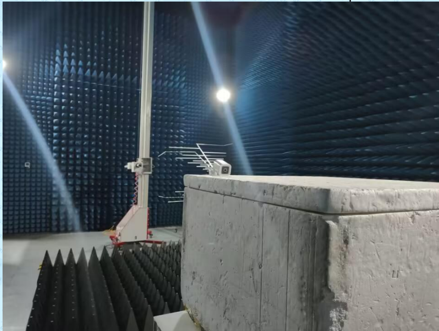
Radiated Emission Above 1GHz Test Setup
