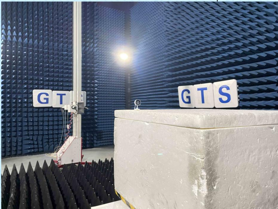
Radiated Emission Above 1GHz Test Setup
