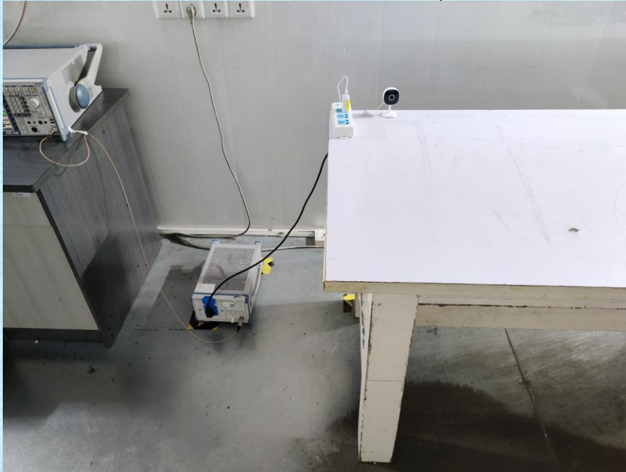
Conducted Emission Test Setup
