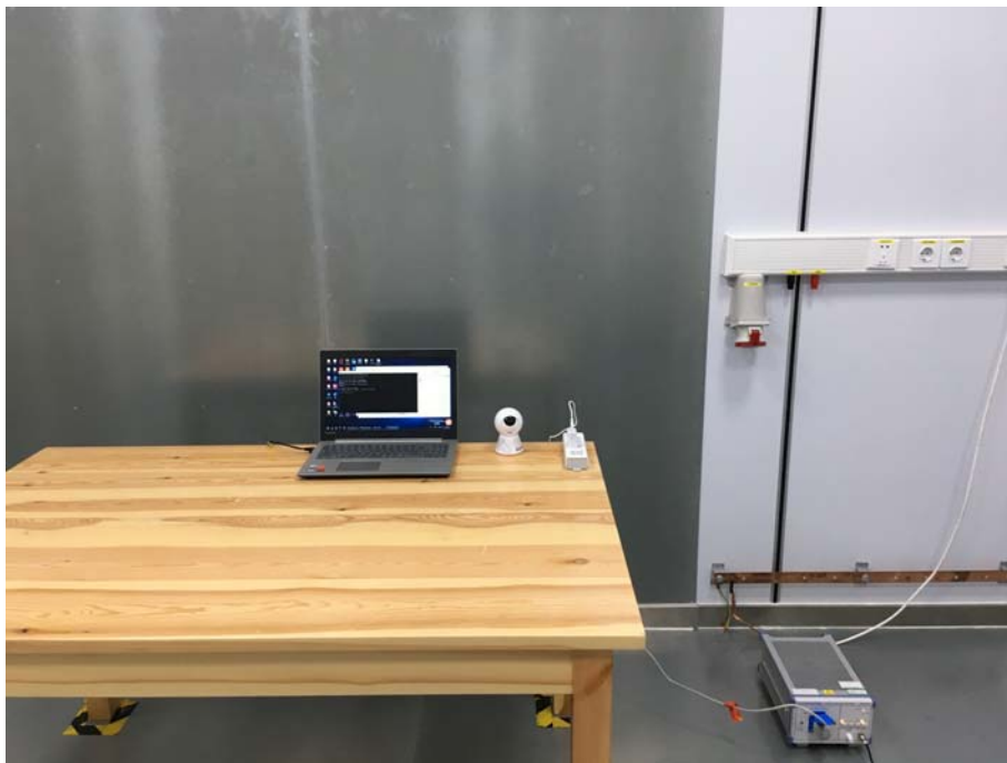
Fig. 4 Power line conducted emission setup photo
