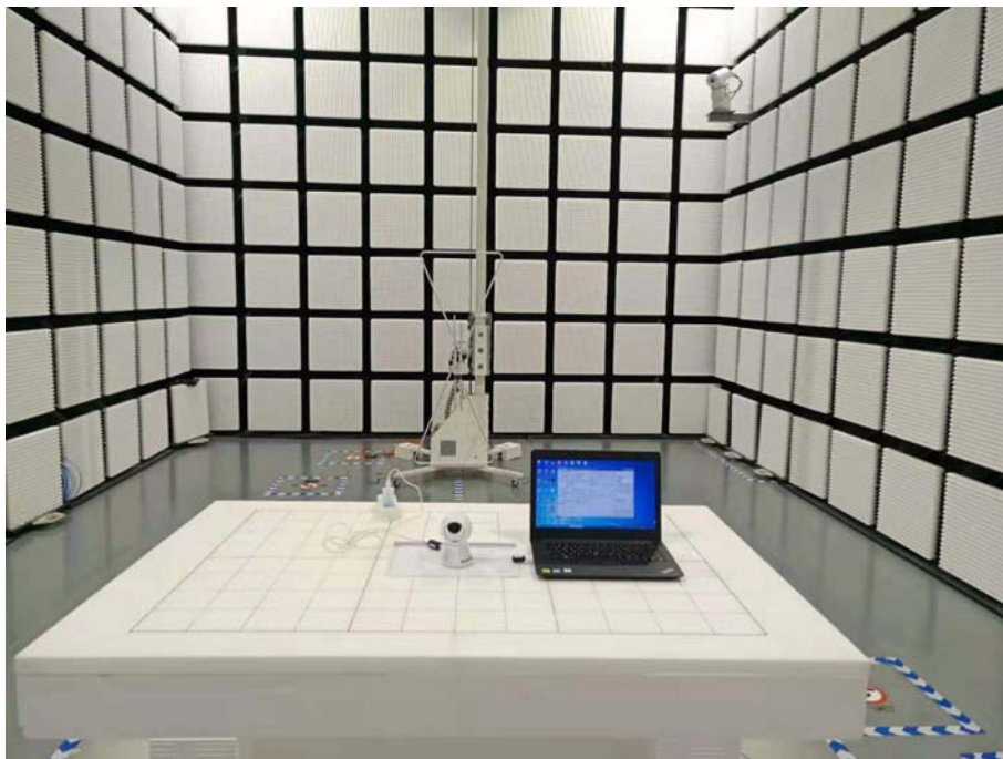
Fig. 2 Radiated emission setup photo(30MHz-1GHz)
