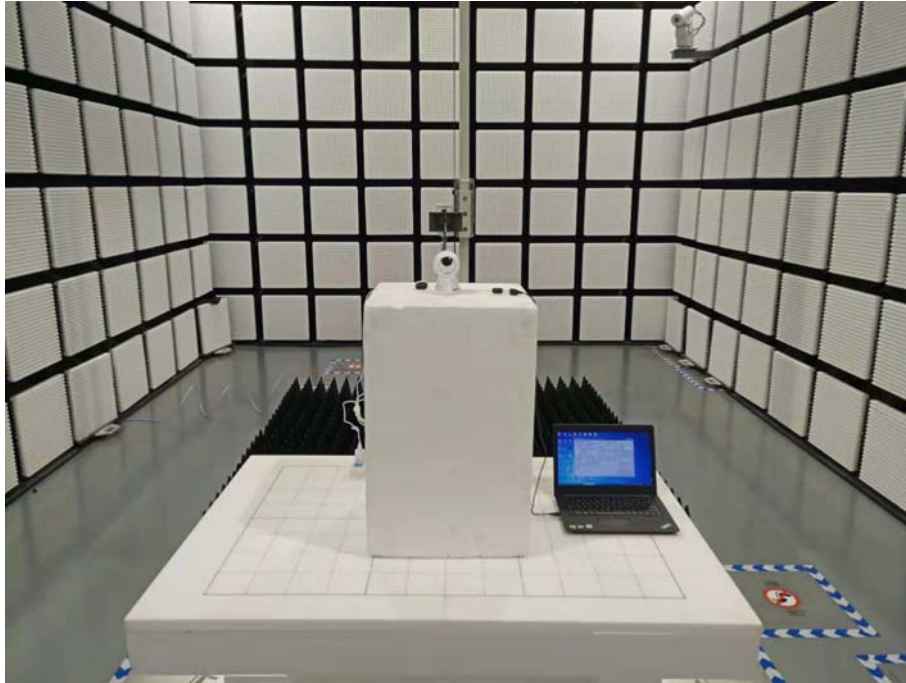
Fig. 3 Radiated emission setup photo(Above 1GHz)
