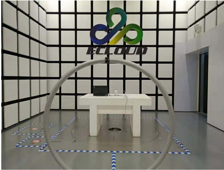
Fig. 1 Radiated emission setup photo(Below 30MHz)
