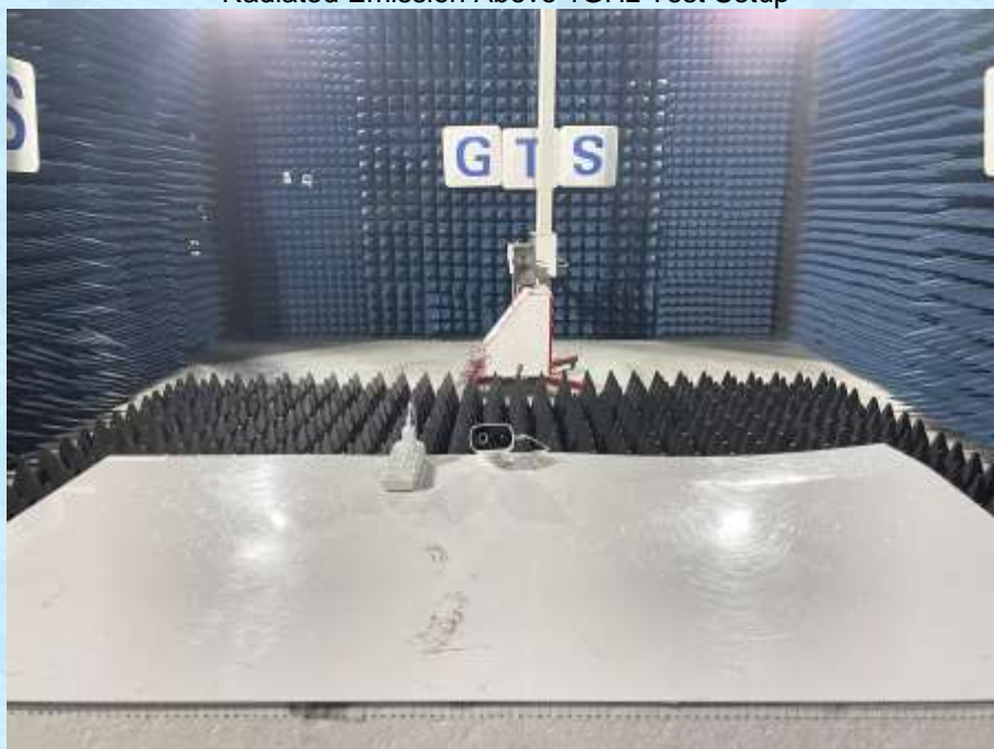
Radiated Emission Above 1GHz Test Setup
