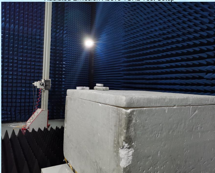
Radiated Emission Above 1GHz Test Setup
