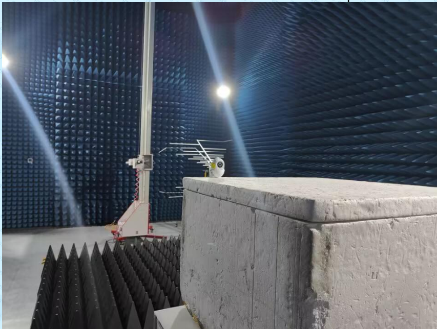
Radiated Emission Above 1GHz Test Setup
