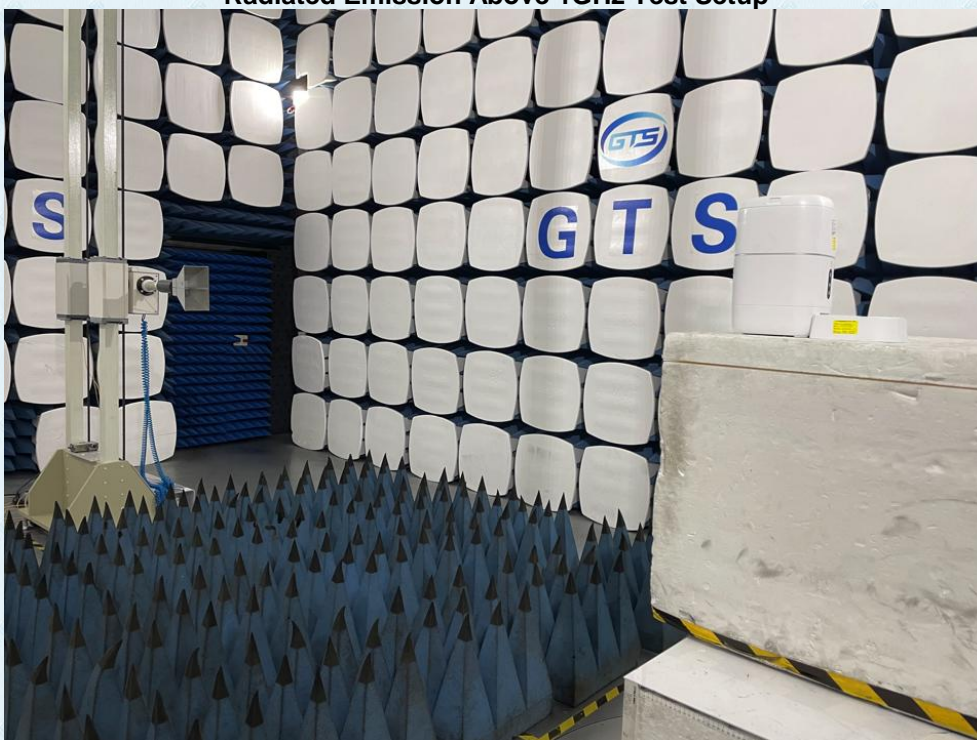
Radiated Emission Above 1GHz Test Setup
