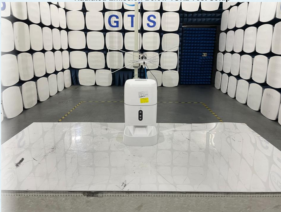
Radiated Emission Above 1GHz Test Setup
