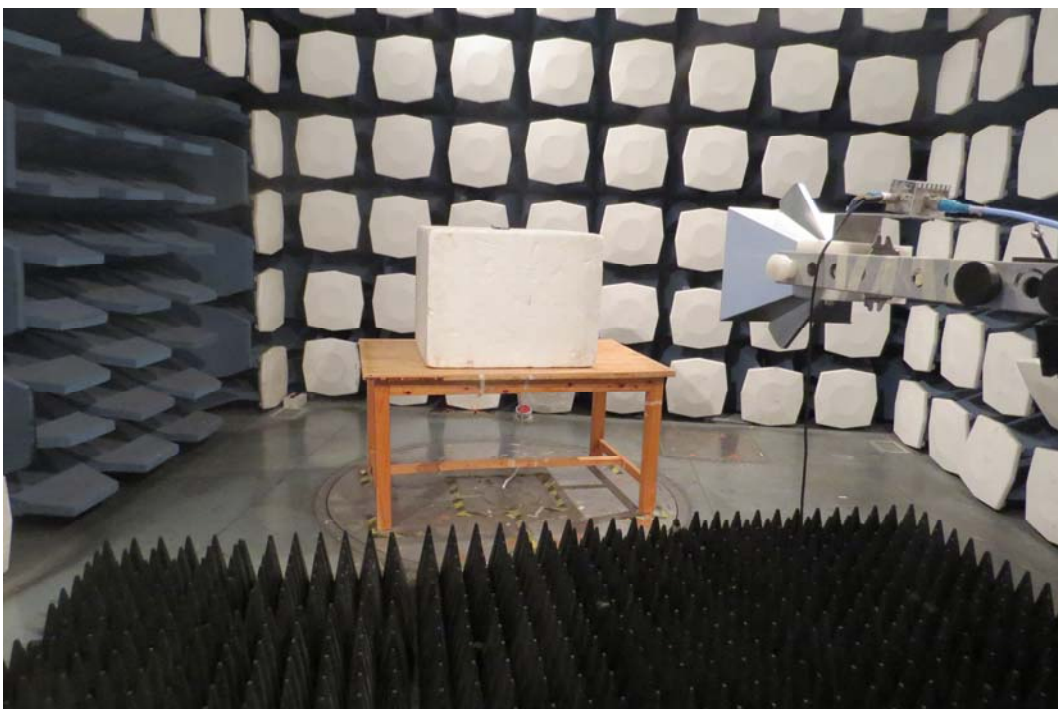
Picture 1: Radiated Spurious Emissions Test setup
