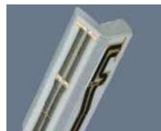
Figure 2 EF3DV3 E-field Probe
