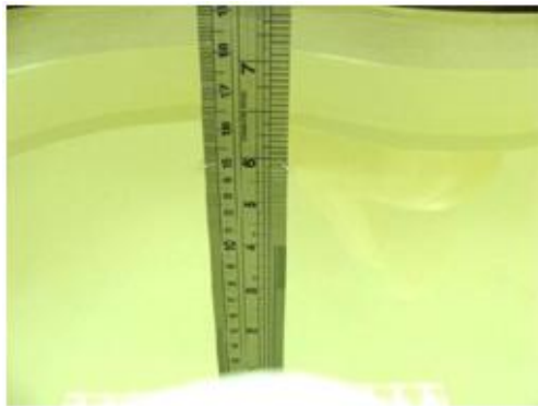
Fig 5.1 Photo of Liquid Height for Head SAR
