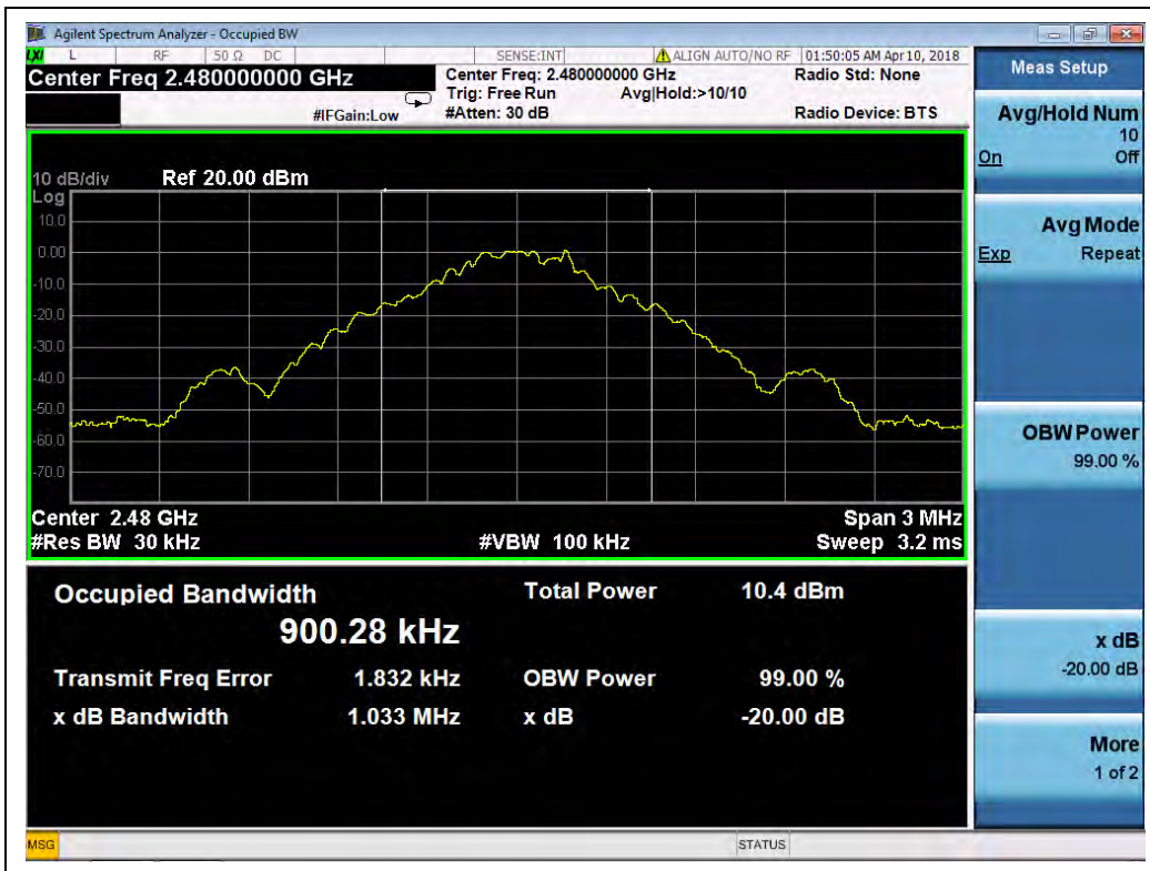
(GFSK, Channel 78, 2480MHz)
