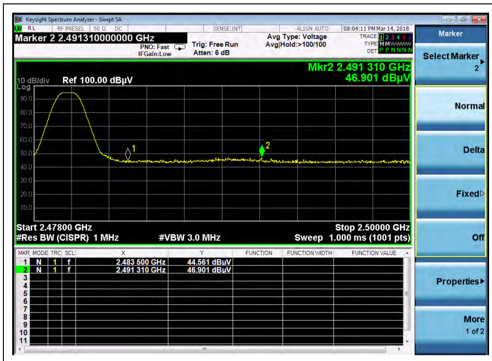
(Channel = 78, PEAK, \pi/4 -DQPSK)
