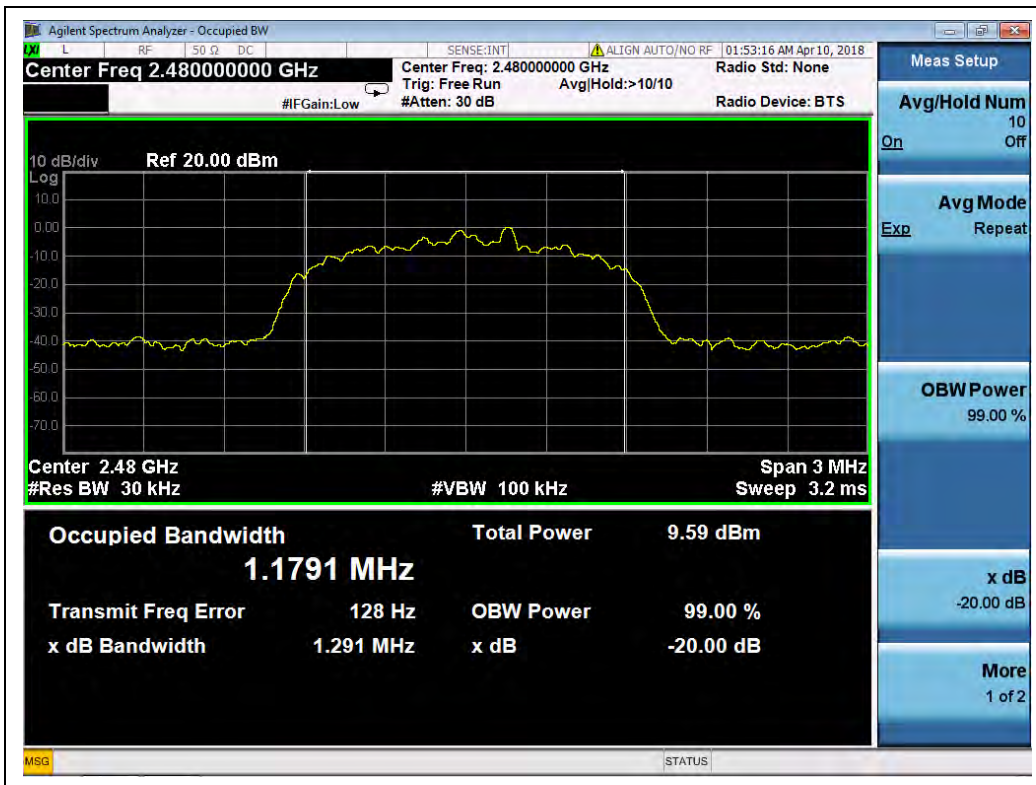
(8-DPSK, Channel 78, 2480MHz)
