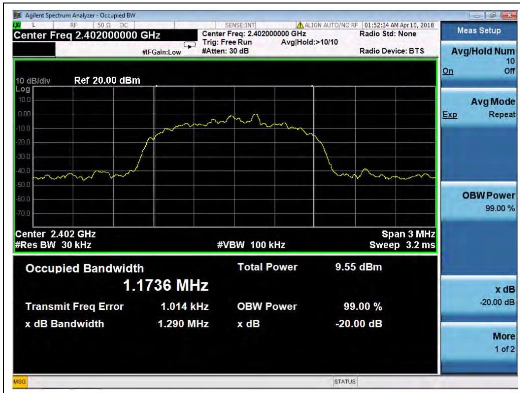
(8-DPSK, Channel 0, 2402MHz)
