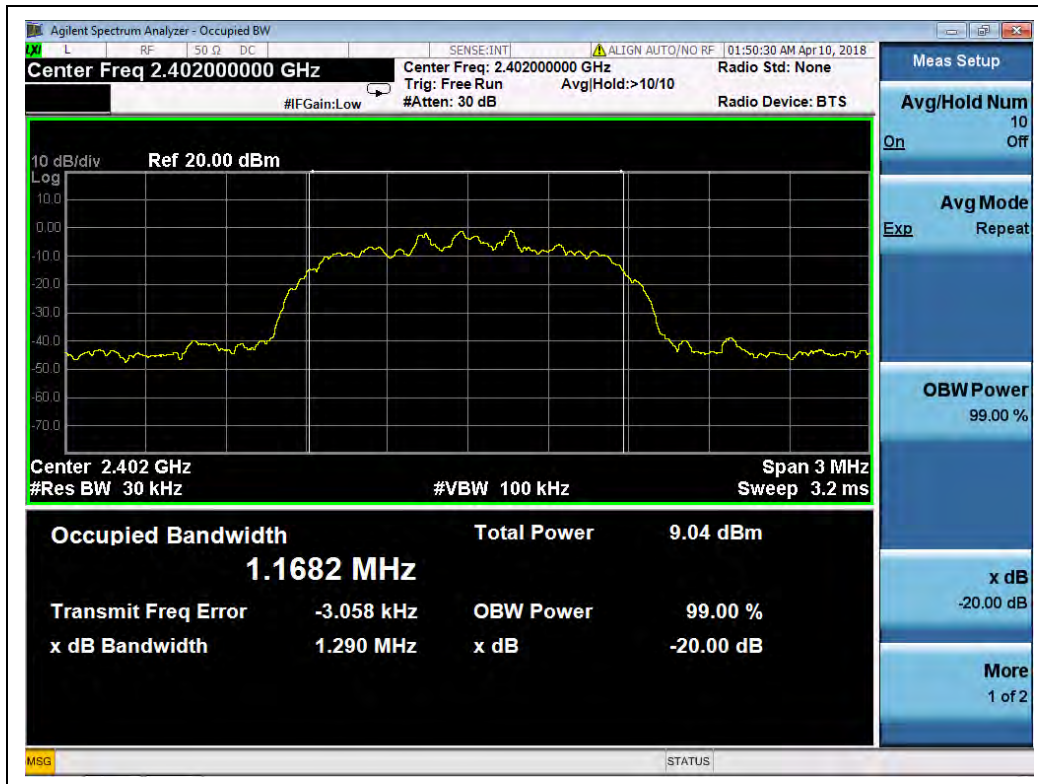
( \pi/4 -DQPSK, Channel 0, 2402MHz)
