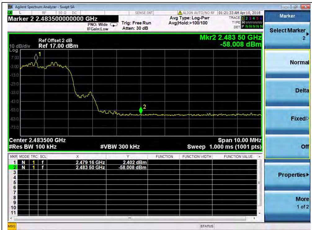
(Channel = 78, Band edge with hopping on, 8-DPSK)
