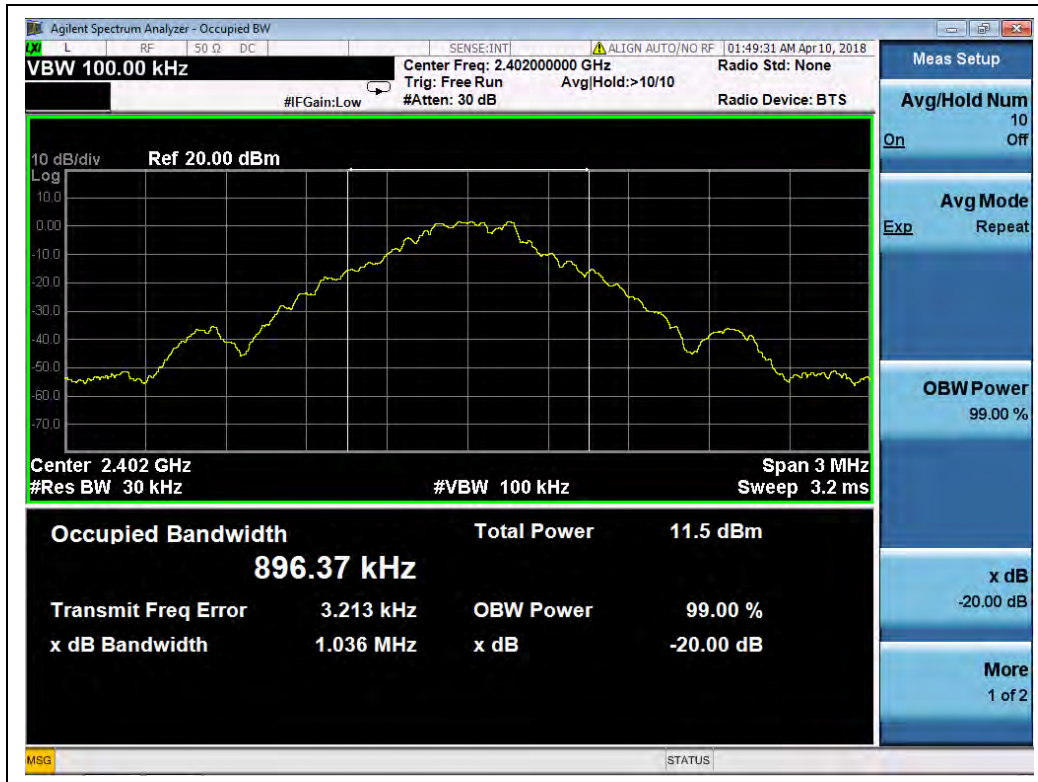
(GFSK, Channel 0, 2402MHz)
