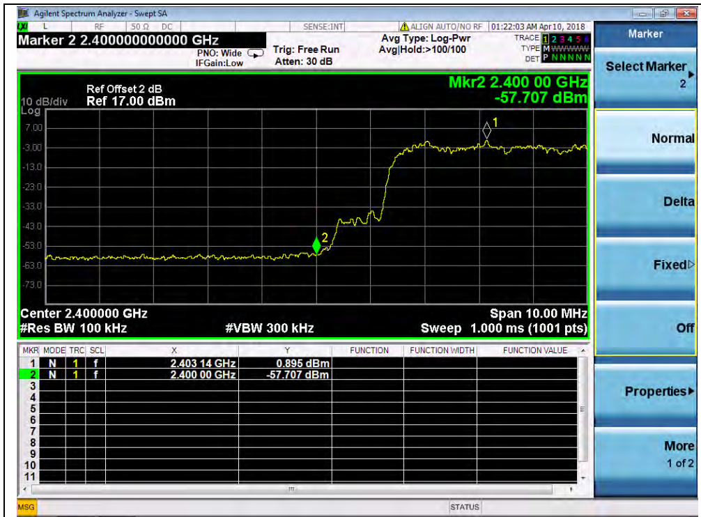
(Channel = 0, Band edge with hopping on, 8-DPSK)
