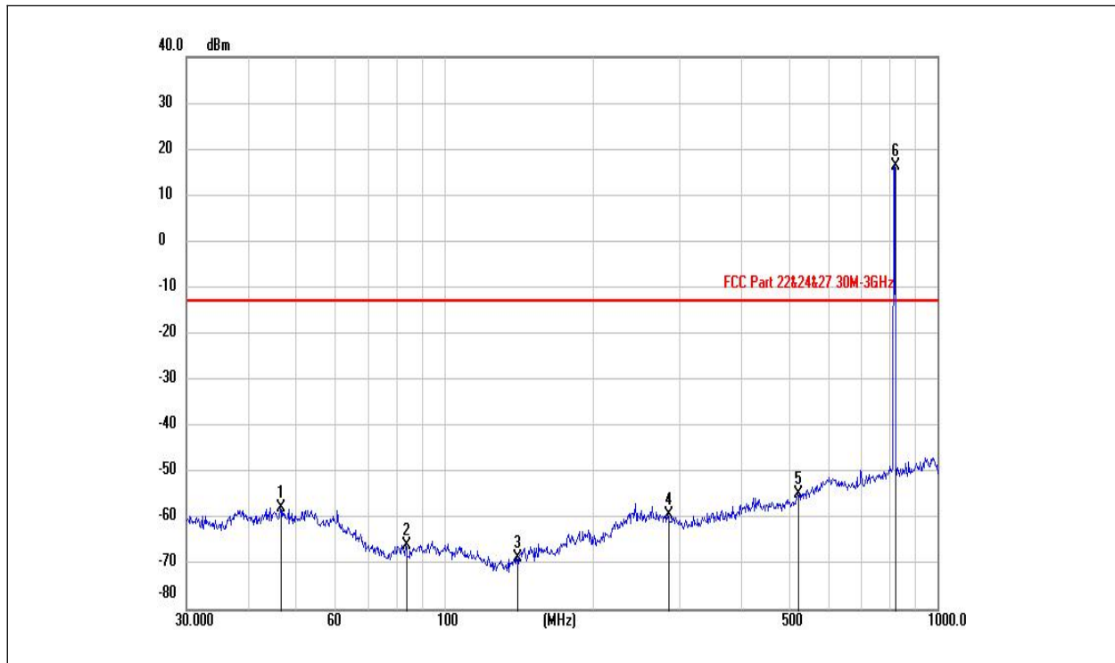
(1XEVD0 Rev 0 BC 10 _ CH 526 _ 30MHz to 1GHz _ Horizontal)
