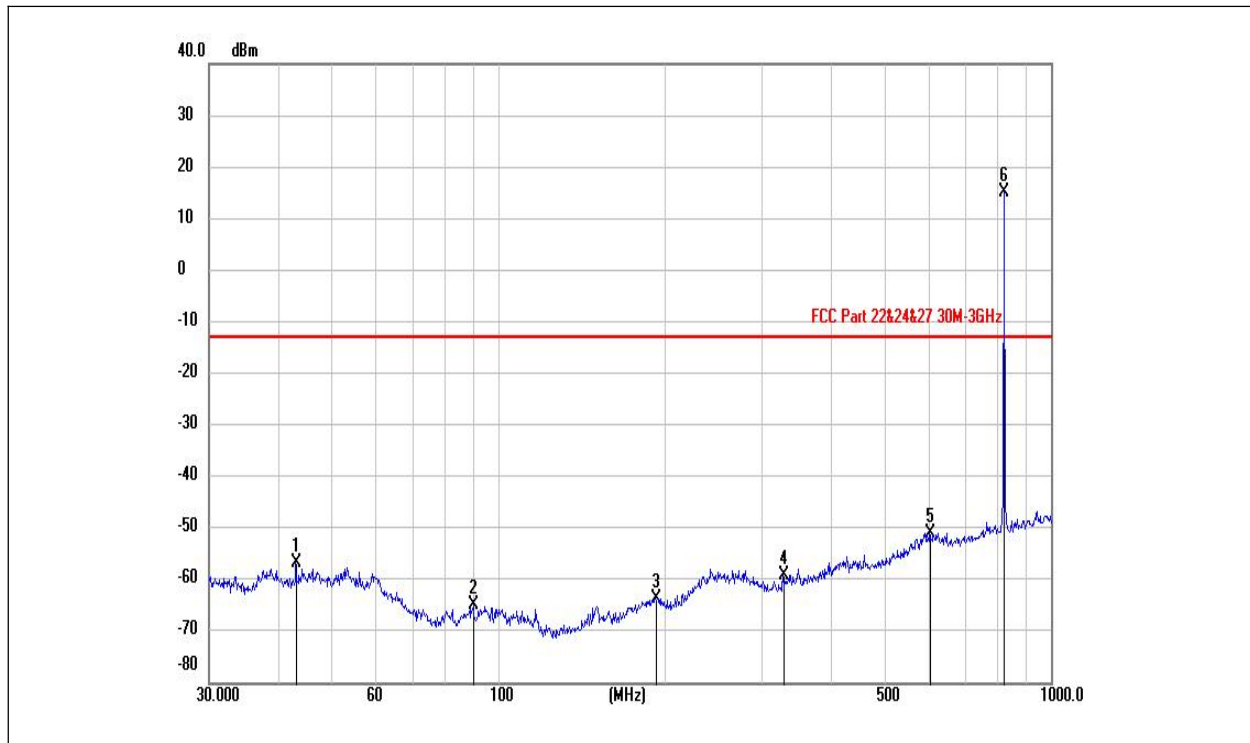
(1XEVD0 Rev A BC 0 _ CH 1013 _ 30MHz to 1GHz _ Horizontal)
