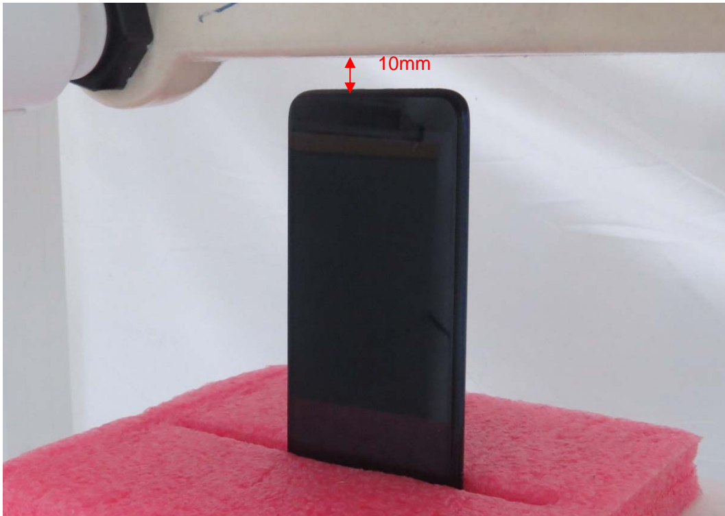
Picture 9: Bottom Side, the distance from handset to the bottom of the Phantom is 10mm
