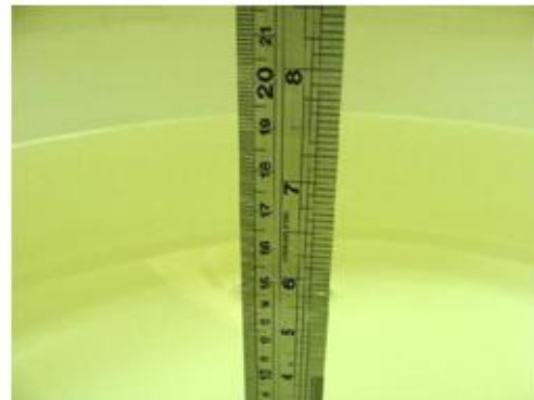
Fig 5.2 Photo of Liquid Height for Body SAR
