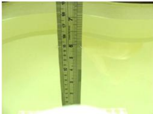
Fig 5.1 Photo of Liquid Height for Head SAR
