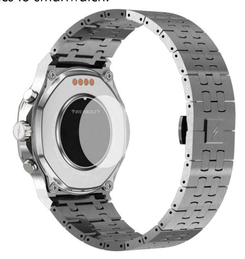
There is a heart rate sensor protector on the sensor, you can take it off before using smartwatch.
