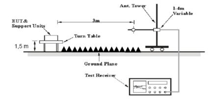
The radiated emissions were performed in the 3 meters distance, using the setup accordance with the ANSI C63.10-2013. The specification used was the FCC 15.205, 15.209, and FCC 15.231 limits.
