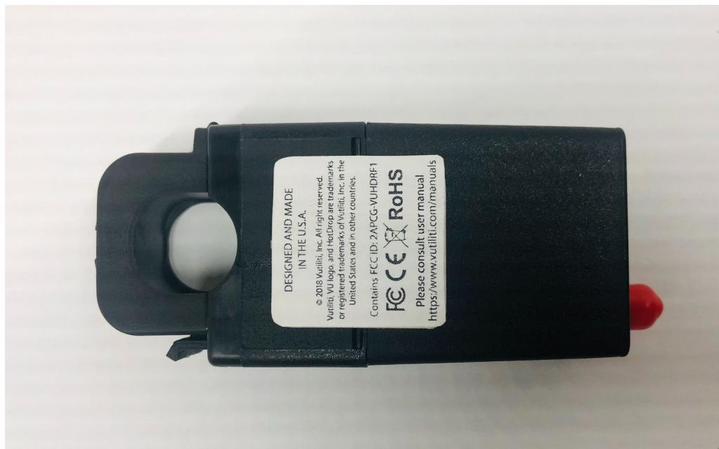
HotDrop Device with NO external antenna attached, internal antenna u.FL may be utilized.
