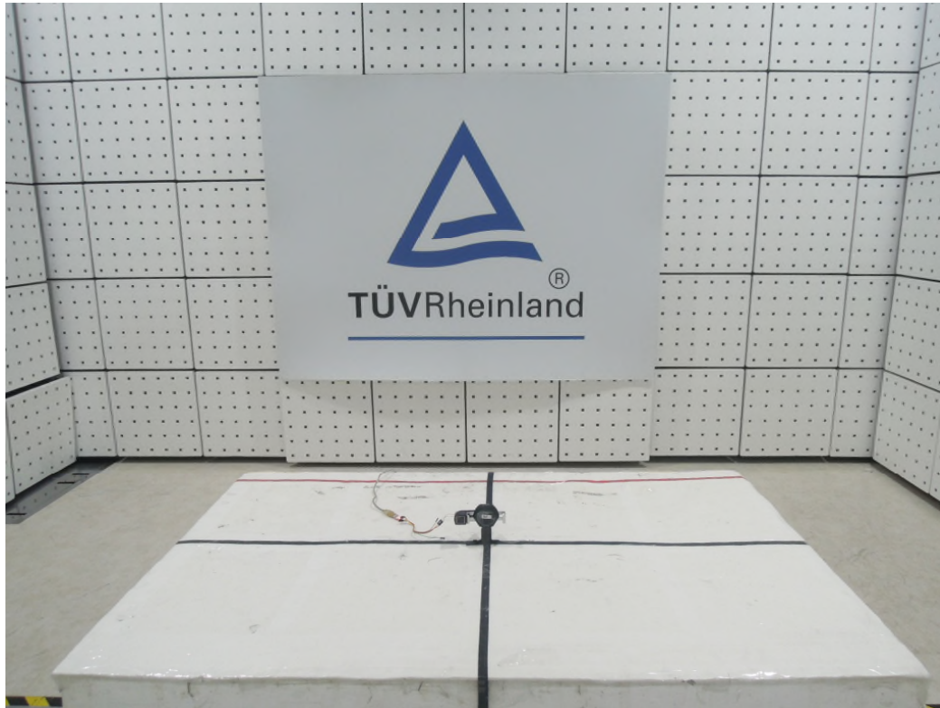
Photograph 2: Set-up for Spurious Emissions (Back View 1)
