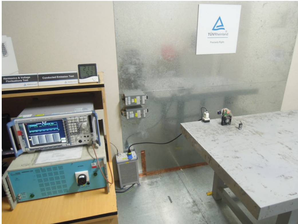
Photograph 6: Set-up for Spurious Emissions, AC Mains (Back View)
