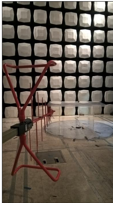
Photograph 2. Radiated Spurious Emissions, Test Setup 2: Below 1 GHz
