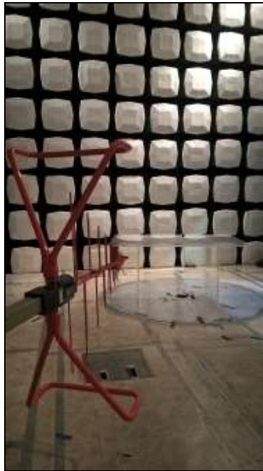
Photograph 2. Radiated Spurious Emissions, Test Setup 2: Below 1 GHz
