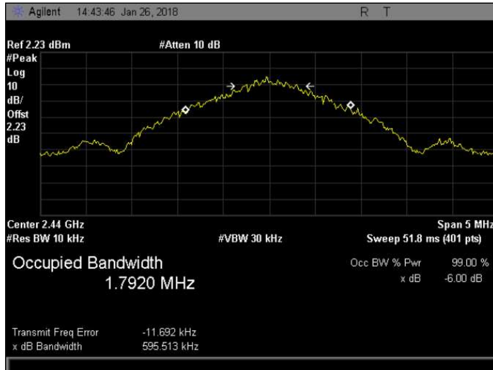
Plot 2. 99% Occupied Bandwidth, Mid Channel
