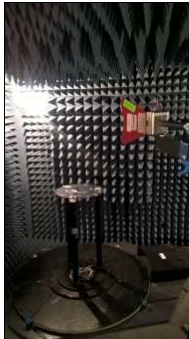
Photograph 1. Radiated Spurious Emissions, Test Setup 1: Above 1 GHz
