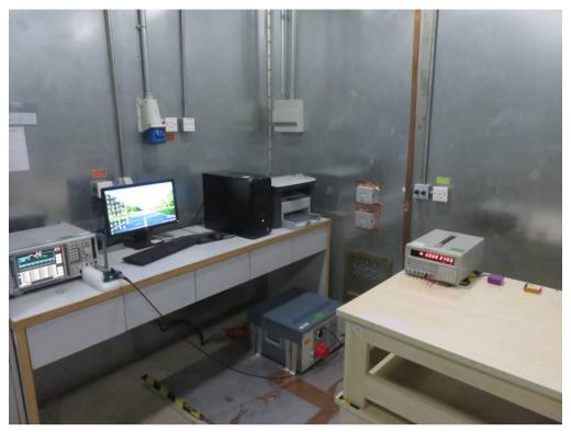
FCC RADIATED EMISSION TEST SETUP
