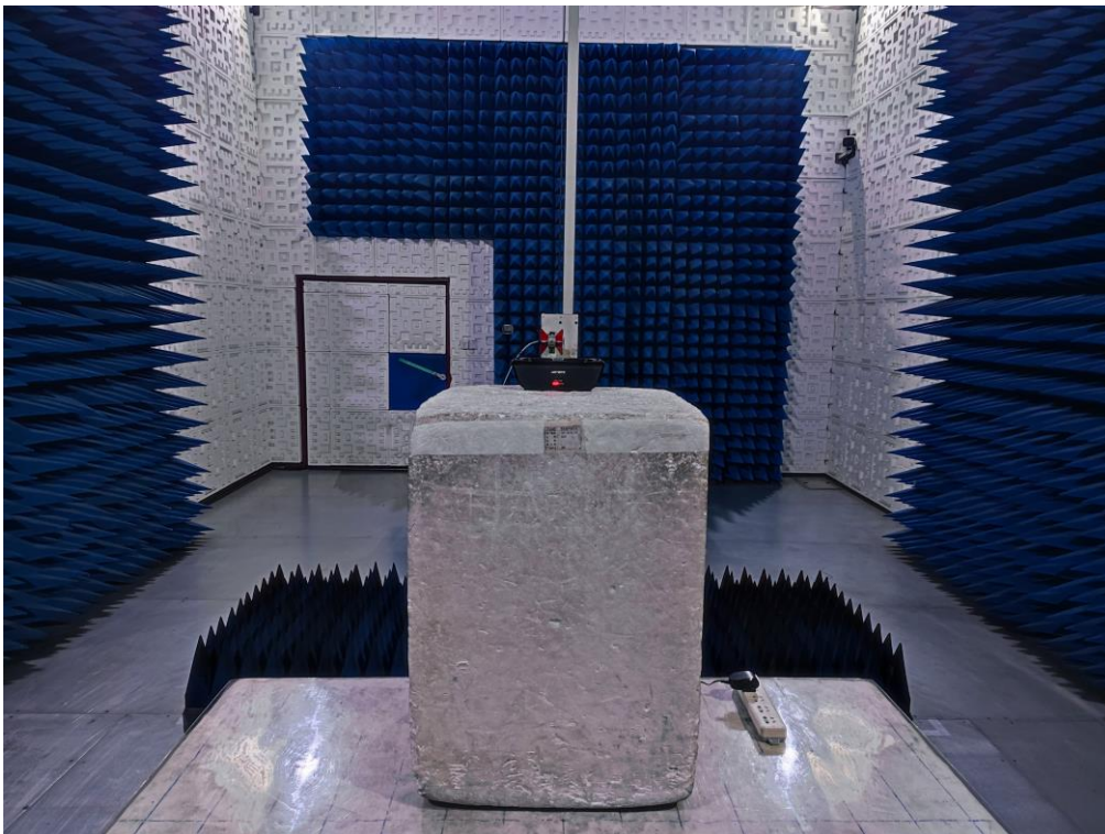
RADIATED EMISSION TEST SETUP ABOVE 1GHZ
