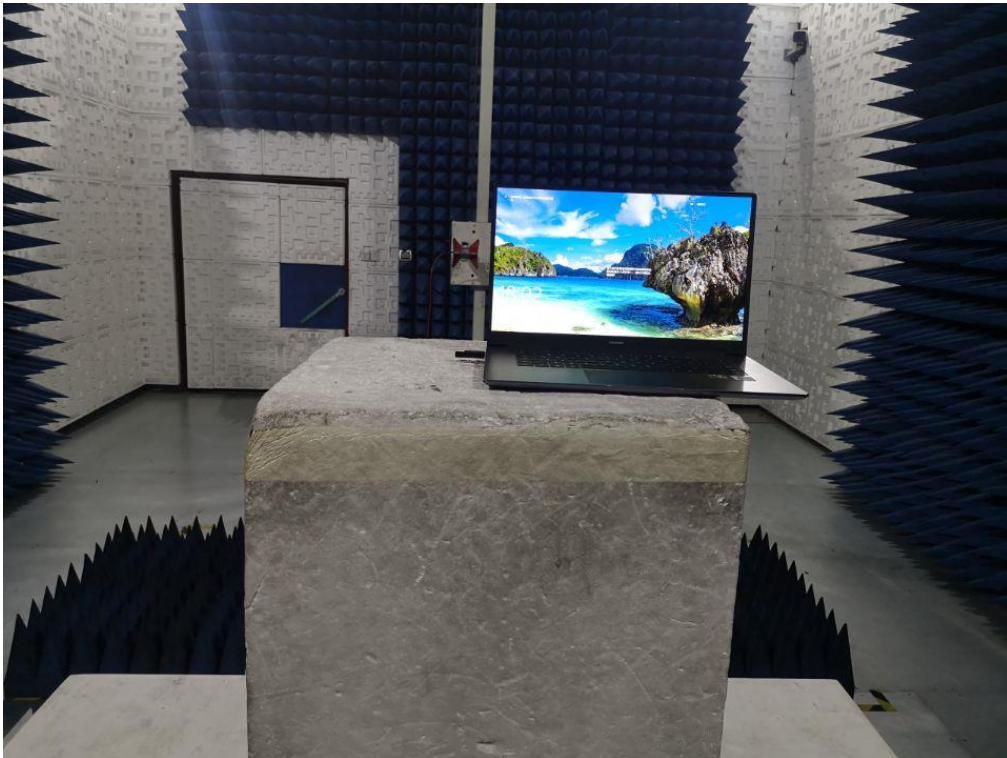
FCC RADIATED EMISSION TEST SETUP ABOVE 1GHZ
