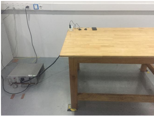
Conducted Emissions Test Setup Front View
