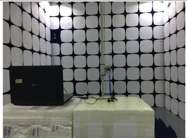
Radiated Spurious Emissions Test Setup Above 1GHz
