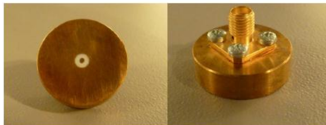
Figure 1 – MVG LIMESAR Dielectric Probe
