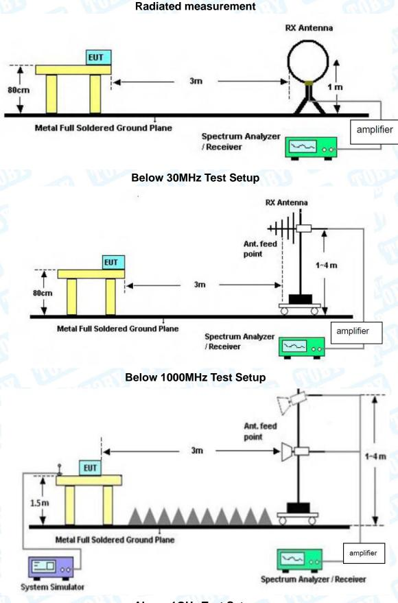
Above 1GHz Test Setup
