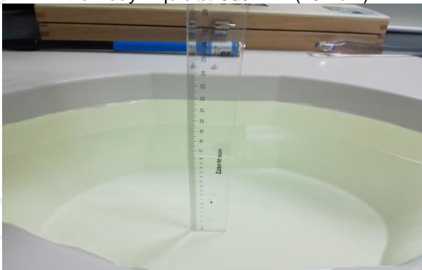
The Body Liquid of 1900MHz (16.4 cm)
