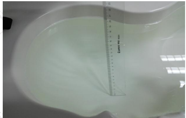
The Head Liquid of 2450MHz (15.6cm)
