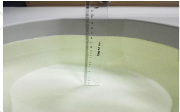
The Body Liquid of 1800MHz (15.2 cm)
