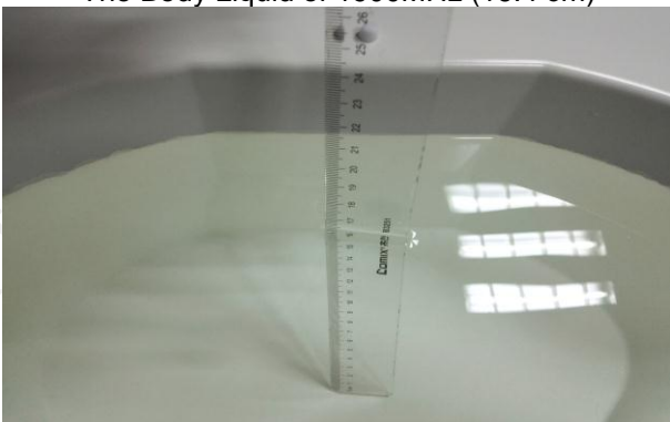
The Body Liquid of 2600MHz (16.5cm)
