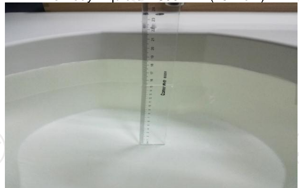
The Body Liquid of 2450MHz (15.3cm)
