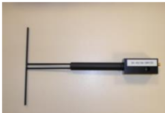
Figure 1 – MVG COMOSAR Validation Dipole
