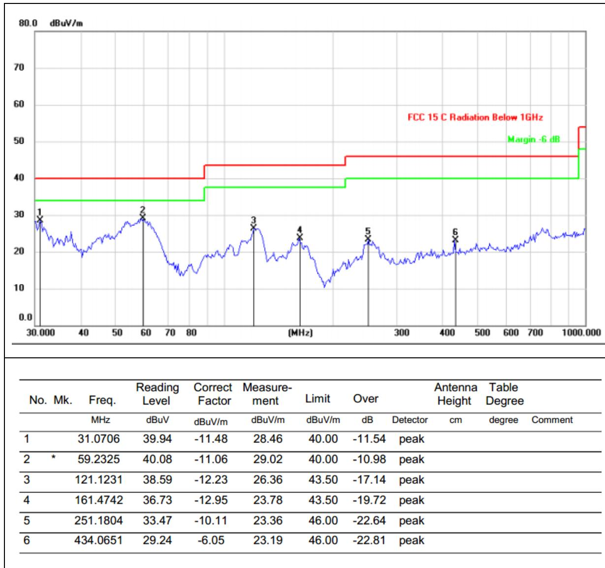
Note1 : Emission Level = Meter Reading + Factor, Margin= Emission Level- Limit, Factor = Antenna Factor + Cable Loss – Pre-amplifier.
