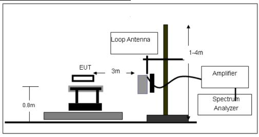
Radiated emission test-up frequency 30MHz~1GHz
