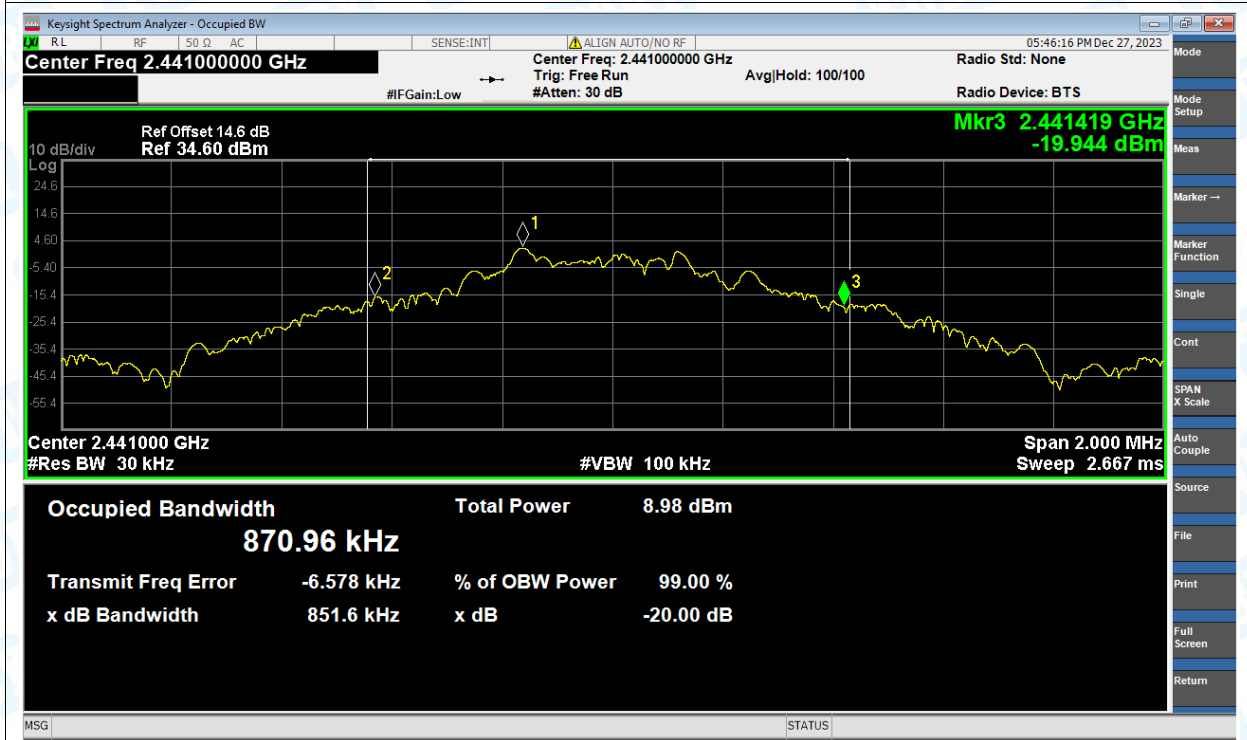
-20dB Bandwidth NVNT 1-DH1 2441MHz Ant1
