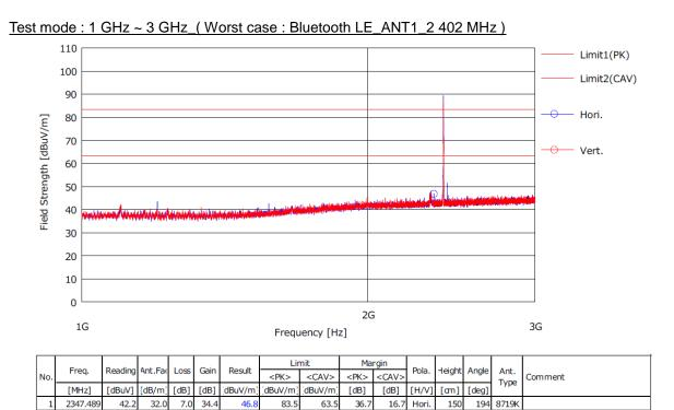
$\begin{array}{lll} \mbox{Note 1:} & \mbox{Measured distance: 1 m} \\ \mbox{Note 2:} & \mbox{Limit: Peak: 83.5 dB} \mu\mbox{V/m} \\ & \mbox{Average: 63.5 dB} \mu\mbox{V/m} \\ \end{array}$
