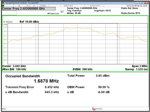
Test mode: Bluetooth LE ANT1 2 440 MHz 6 dB Bandwidth, Occupied Bandwidth
