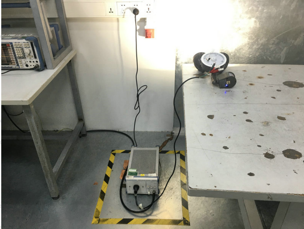
Photo of Conducted Emission Measurement
