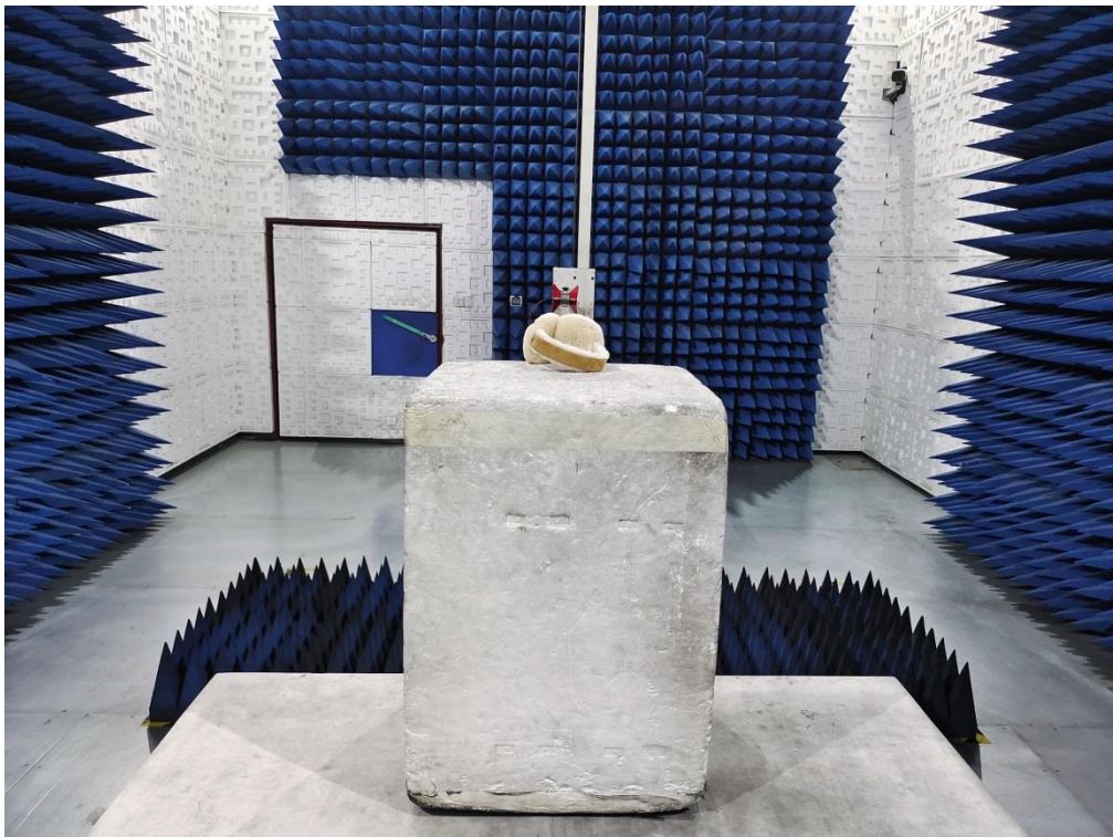
RADIATED EMISSION TEST SETUP ABOVE 1GHz
