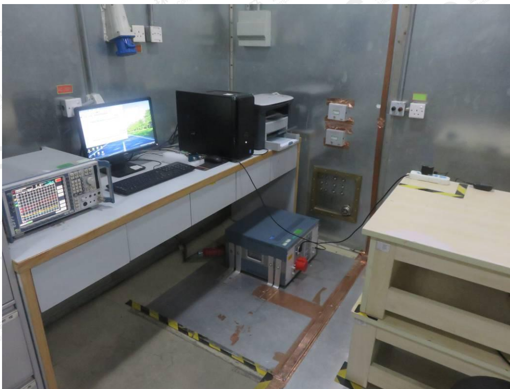
FCC RADIATED EMISSION TEST SETUP
