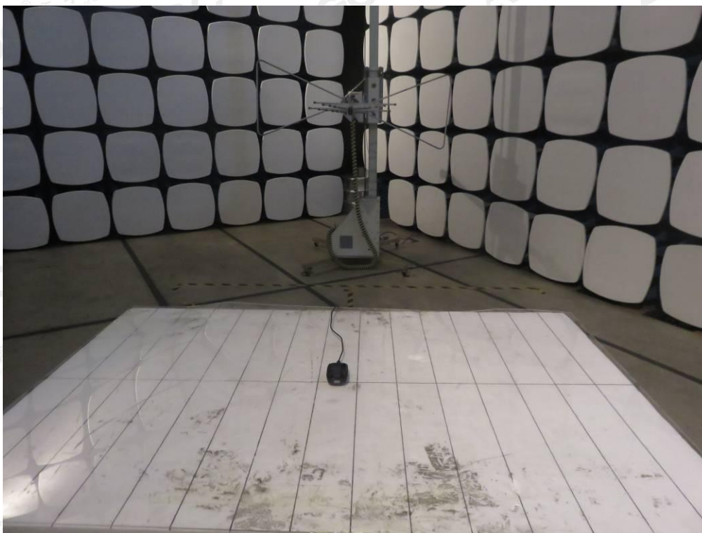
FCC RADIATED EMISSION TEST SETUP
