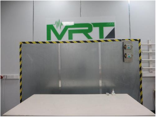
Test Mode 1 Description: Back View Conducted Emission Test Setup for Power Port
