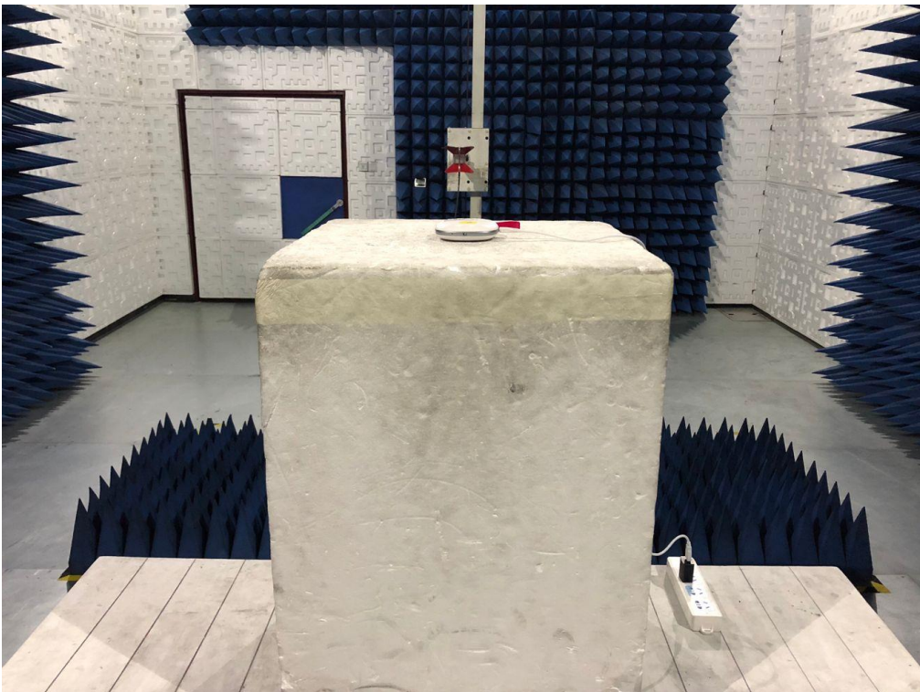
RADIATED EMISSION TEST SETUP ABOVE 1GHZ
