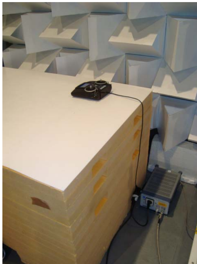
Figure 4 EUT / test set up - spurious conducted emissions
