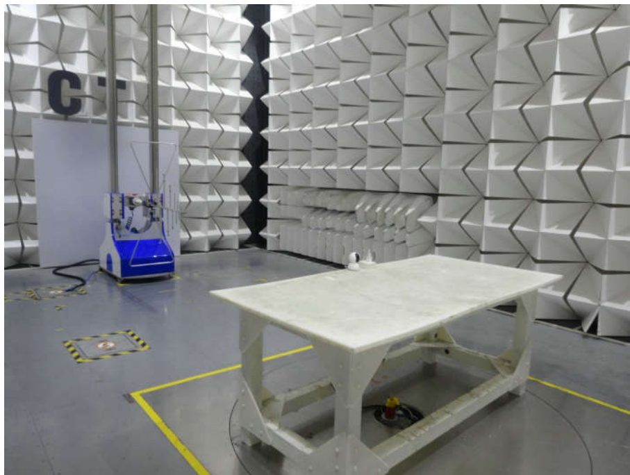
Radiated spurious emission Test Setup-2(30M-1G )
