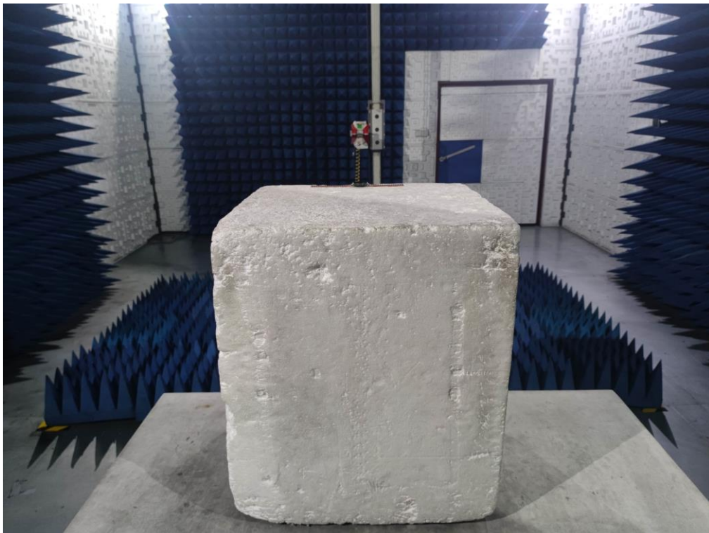
RADIATED EMISSION TEST SETUP ABOVE 1GHz
