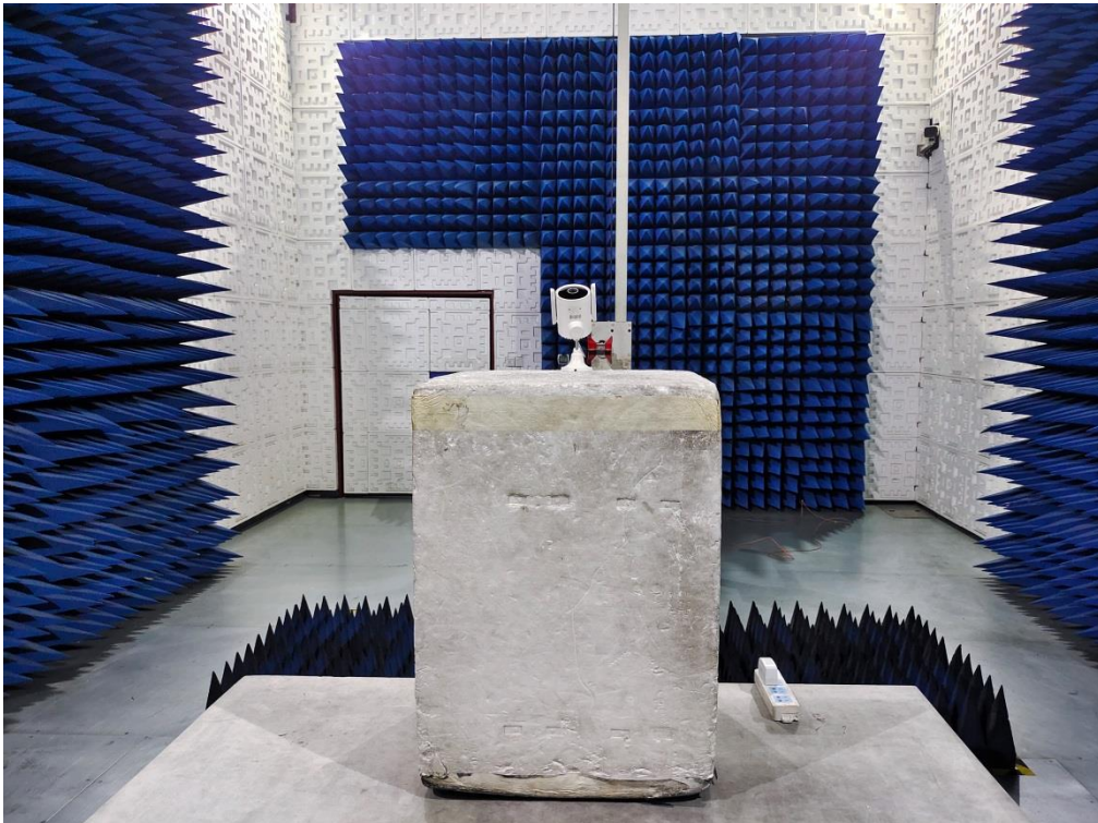
FCC RADIATED EMISSION TEST SETUP ABOVE 1GHZ
