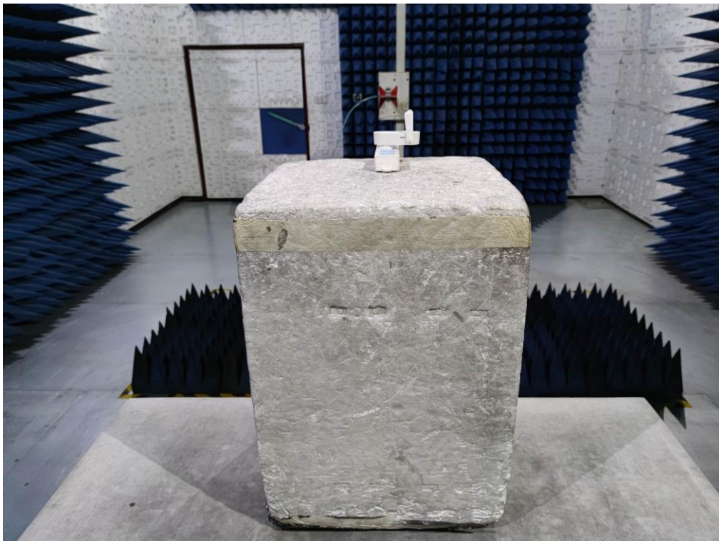
RADIATED EMISSION TEST SETUP ABOVE 1GHz
