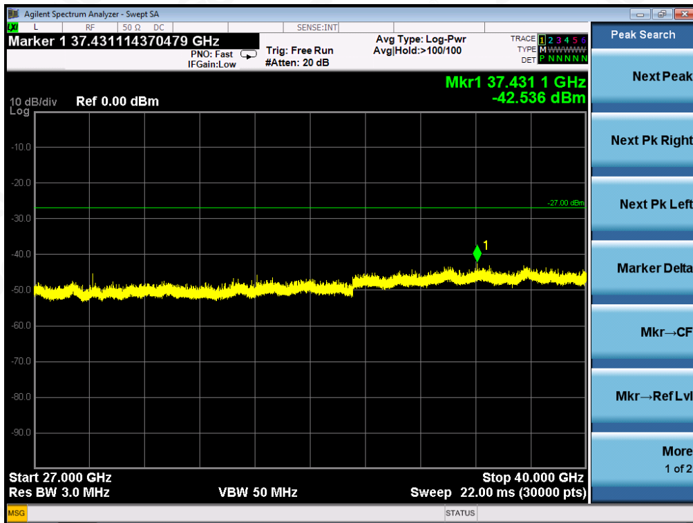
TEST PLOT OF OUT OF BAND EMISSIONS FOR MODULATION IN 5320MHz
