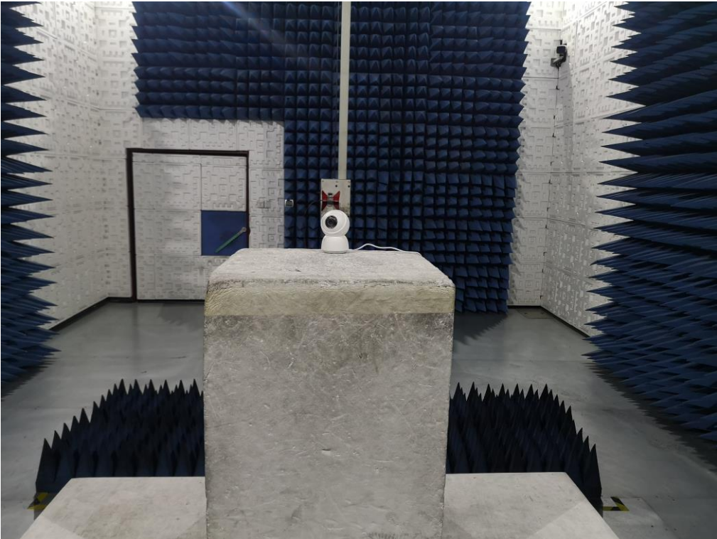
FCC RADIATED EMISSION TEST SETUP ABOVE 1GHZ
